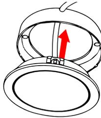
2. Route fixture wires through center of housing toward power supply location; position wires in housing notch.
