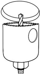
1. Use a hole saw and cut a 2-1/2" hole through mounting surface.
