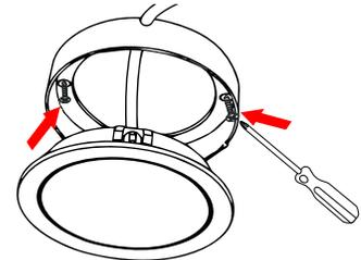
3. Secure housing to mounting surface with 2 screws, included.
