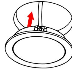
3. Route fixture wires through the hole toward power supply location.
